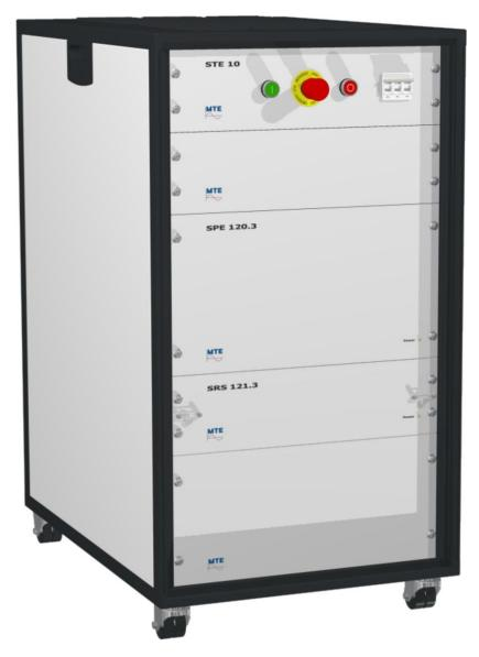
The SPE System is an electronic voltage- and current power source and a meter supply unit (phantom load) for testing electricity meters or for testing other devices which use current or voltage. In addition to the generation of standard test values, the meter test equipment offers the following options:
